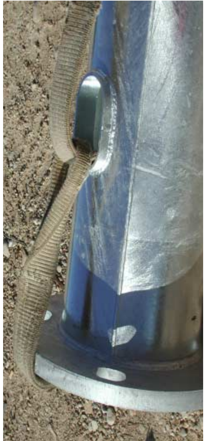
Figure 56 - Bottom Lifting Point
